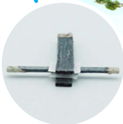
The transistor used wood from a balsa tree (left). Natural channels in the wood were enlarged (center) and coated with an electrolyte gel (shown in blue). The result was a piece of wood that could conduct electricity (right).
