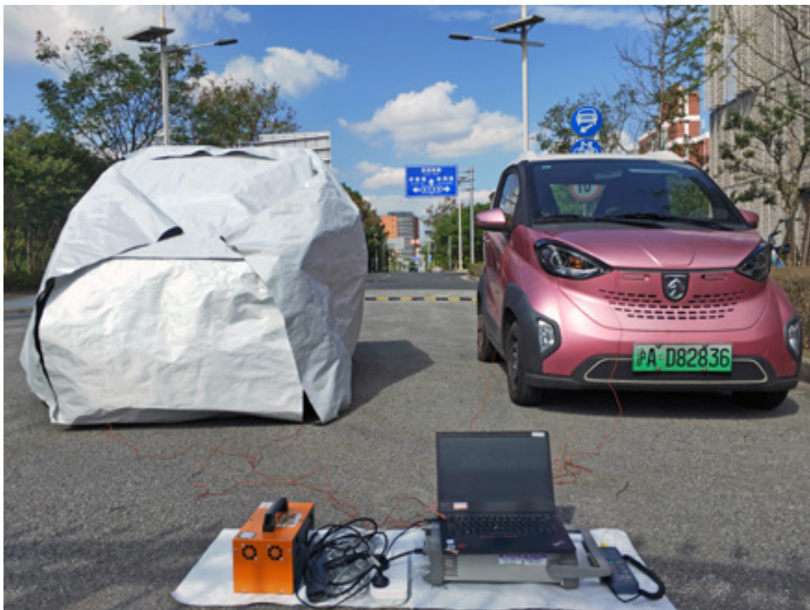
Draping the new fabric over one car (left) kept its inside temperatures up to 28 degrees Celsius (50 degrees Fahrenheit) cooler than an uncovered car (right).
